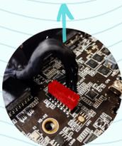
OBS: ANTES DE RETIRAR A PLACA MÃE, DESCONNECTE O CABO DO PAINEL FRONTAL PUXANDO PARA CIMA.
